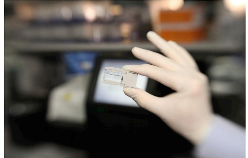
Flow cell for the Illumina MiSeq sequencer.
